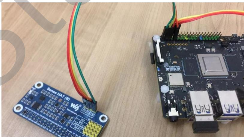
**Figure 1-2 Connect Sense Hat (B) to the 40-Pin Header**
