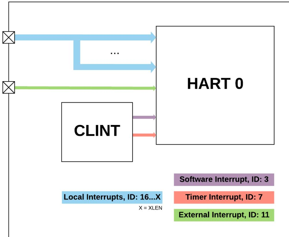
Figure 3: CLINT Block Diagram for Machine Mode
