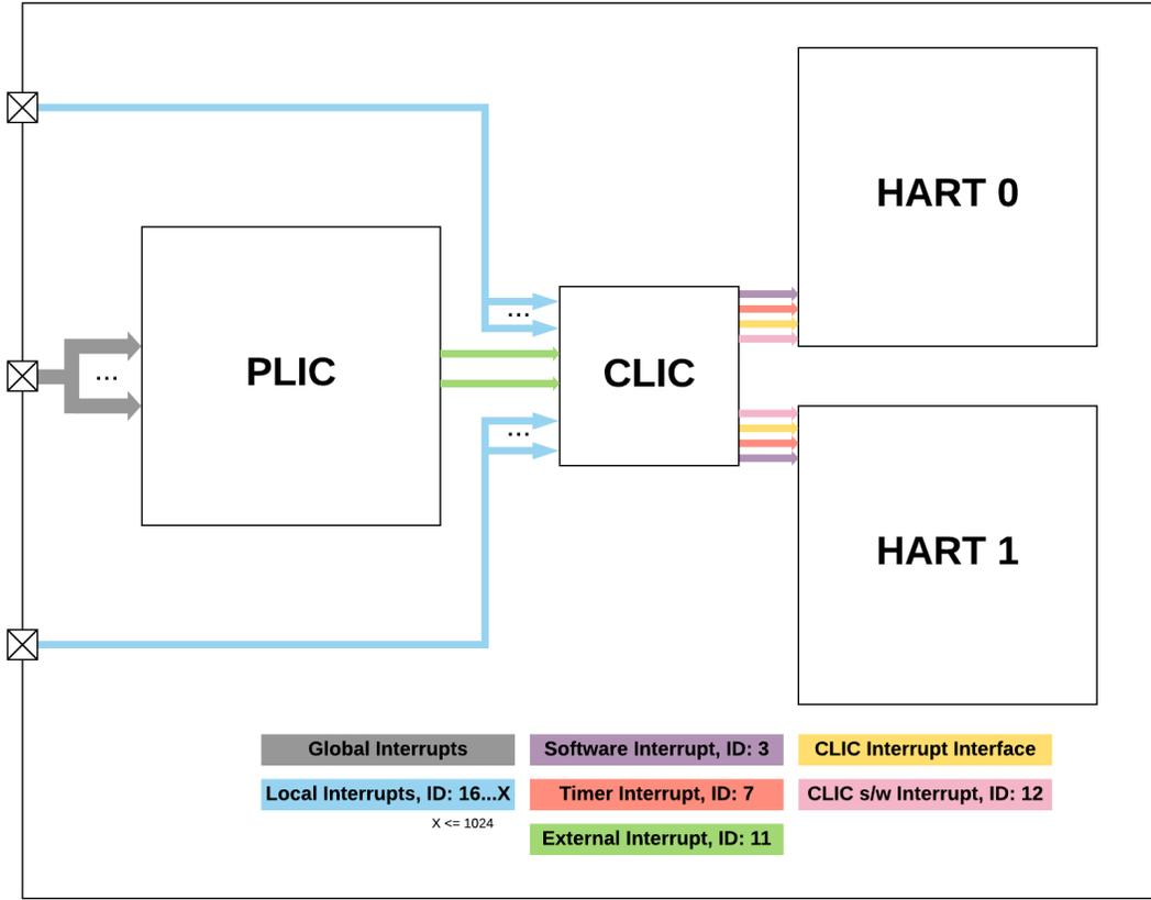
**Figure 9:** PLIC + CLIC Block Diagram for Machine Mode
