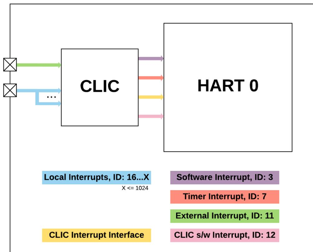
**Figure 7:** CLIC Block Diagram for Machine Mode
